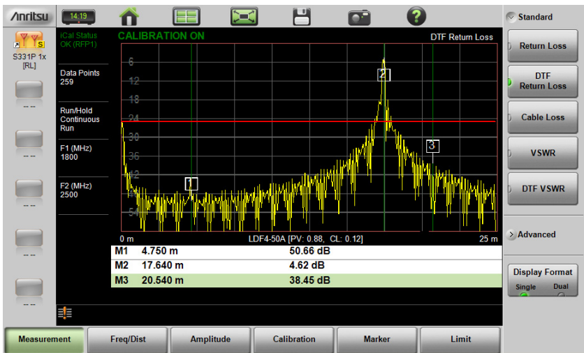
Figure 3-14. Failing DTF Return Loss Measurement (Load at 20.54 m)
