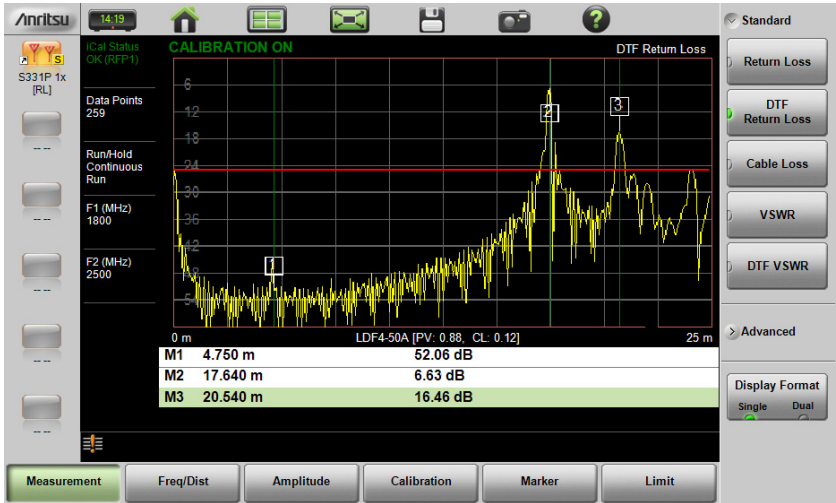
Figure 3-13. DTF Return Loss Measurement (Antenna at 20.54 m)
